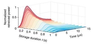
**Fig. 5** 1s long light storage. Light storage for up to t=1s of short ( $\tau_p=5.5$   $\mu$ s) signal pulses
